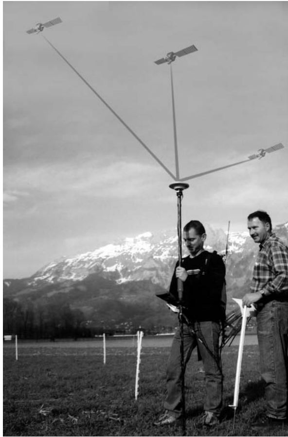
Fig. 4: Using the Leica GS20, the landscape architects recorded vegetation data for the Data model in three dimensions.
