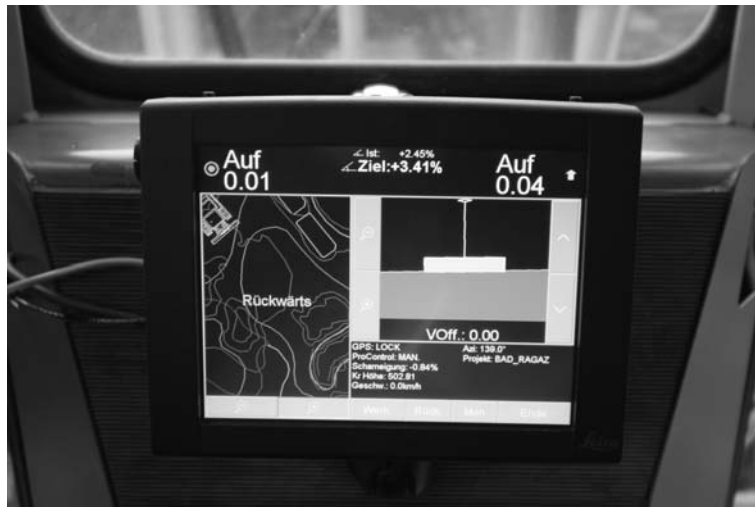
Fig. 5: In the driver's cabin one can see the terrain model on the machine operator's Display unit. The planning data is combined with the clear guidance data from real time GPS positioning providing the machine operator with all the necessary details for excavation, graphically and digitally, accurate to within a centimetre – more quickly, more comprehensively and more precisely than marker poles.
